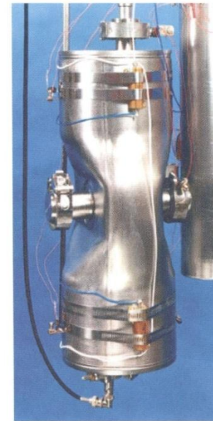
Figure 4.26 350-MHz \beta = 0.12 coaxial half-wave resonator with a single loading element (courtesy of J. R. Delayen, Ref. 33).
